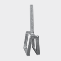
Free standing ridge bracket unit. Height 400mm. Requires 2 x 250mm x 250mm concrete slabs (Obtain locally)
